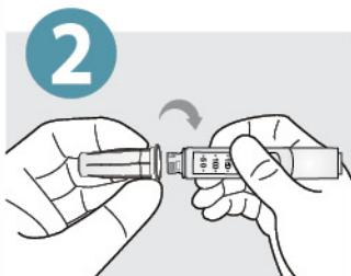
2. Holding the shield, align the end of needle hub with the refill and screw it clockwise onto the injection pen.
